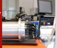
Sub-Assembly Test and measurement of slip rings at subassembly stage in the manufacture of drones, periscopes, wind turbines, medical instrumentation, and defence applications
